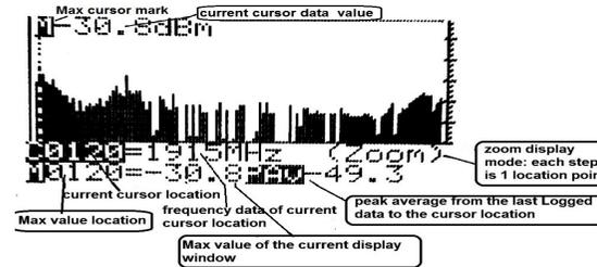
(3) **To move the cursor** in the display window: The cursor in the display window is pointing to the cell address of the Buffer memory. The 1024 signal level and frequency data stored in Buffer memory can be displayed by Moving the cursor with "<" and ">" button in the Data Logging view mode. Push and hold down the "<" or ">" button will fast move the cursor.
