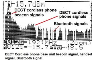
**Duty Cycle of the digital RF burst signal:**
