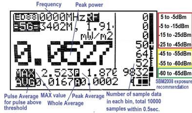
(16) **5G indicator:** When a 5G network frequency signal (5G channels n5, n71, n77, and n78) is detected, the <5G> mark on the display will be displayed as <5G> with reverse color. The frequency counter display is capable of operating at frequencies of up to 4.2GHz.
